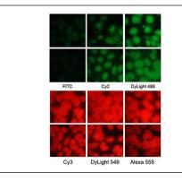
Fig.1. DyLight fluorescent dyes are a new family of dyes with improved brightness. DyLight 488-antibody conjugates are brighter than Cy2 and FITC conjugates and similar in brightness to Alexa Fluor 488 conjugates. DyLight 549-antibody conjugates shows brighter influoresence than TRITC conjugates. Also, DyLight 594-antibody conjugates are noticeably brighter than Alexa 594 conjugates, and much brighter and more water soluble than Texas Red conjugates.
