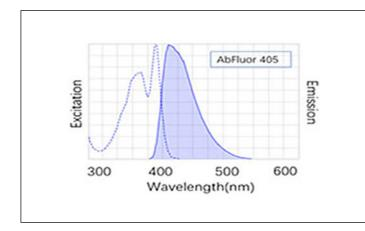
Fig. AbFluor™ 405 (λEX/λEm: 404/431 nm) is super alternative to Alexa Fluor 405, Cascade Blue dye and DyLight 405.
