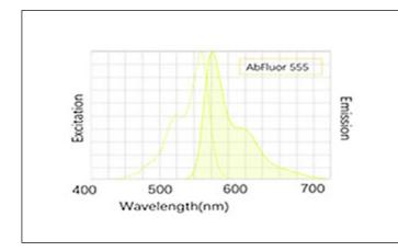
Fig. AbFluor™ 555 (λEX/λEm: 555/565 nm) is a bright and photostable fluorescent dye which is super alternative to Cy3, Tetramethylrhodamine, Dylight 549 and Alexa Fluor 555.
